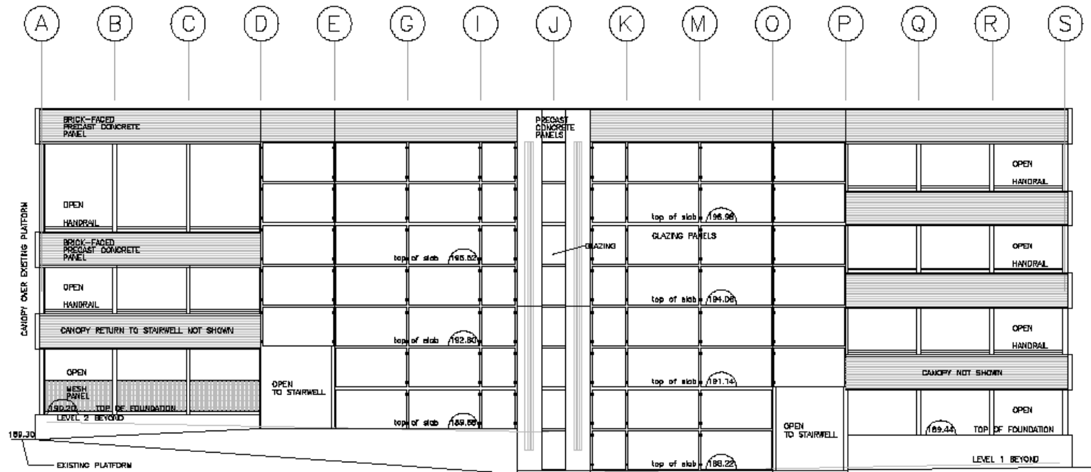
GLAZING PANELS: 13mm TEMPERED GLASS RAINSCREEN. GLASS PANELS SECURED TO COLUMNS WITH PRE-ENGINEERED CLIPS. 30mm AIR SPACE BETWEEN PANELS.
